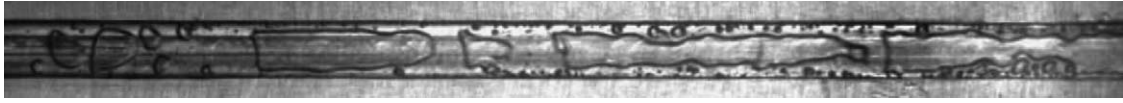
Fig. 9. Typical steady boiling with two characteristic bubble diameters in a 0.5 \times 4 \times 200 \text{ mm}^3 minichannel ( \dot{Q}_M = 240 \text{ kg m}^{-2} \text{ s}^{-1} , Q_W = 3.3 \times 10^4 \text{ W m}^{-2} ).
