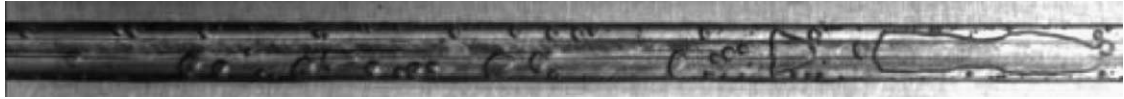
Fig. 5. Picture of typical steady boiling occurring in a 0.5 \times 4 \times 200 mm minichannel ( Q_M = 240 \text{ kg m}^{-2} \text{ s}^{-1} , Q_W = 3.3 \times 10^4 \text{ W m}^{-2} ).
